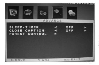
**Sleep Timer:**Select the sleep time to put automatically the TV in standby mode. Timer can be selected as 5min/10min/ 15min/30min/45min/60min/Off. Also you can select the sleep time by pressing SLEEP button repeatedly on the remote control **CLOSE CAPTION:**Select the caption and TEXT modes(CC1,CC2,CC3,CC4,TT1,TT2,TT3, TT4,OFF).
